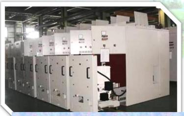
DC Switch gear for Taipei MRT System (DC 750V 6,000A) © Fortune Electric since 1969.
