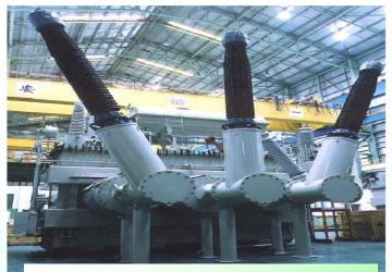
262kV 65MVA Transformer to Japan
